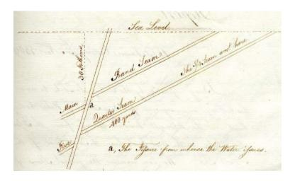
The above circumstances induced us to think......it more than probable, that the Feeder of Water was issuing from the Five Quarter Coal Waste, for as it was allowed that, the Coal of that Seam was pervious, it was by no means unlikely that the Fissure of the Dyke should be equally so.
