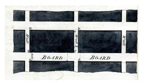
The Workings of a Coal Pit form a Succession of Parallelograms, as represented in the annexed Sketch, each of which from **a**, to **c**, is called a Winning, and from **a**, to **b**, a Pillar. The Excavation **e**,**f**, is called a Wall, and the Excavation **c**,**d**, is called a Board.
