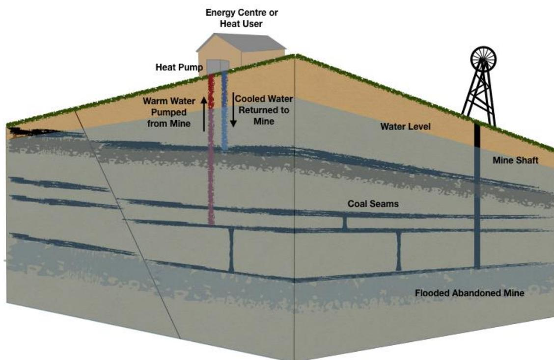
*Schematic Diagram of a minewater heat pump system*
