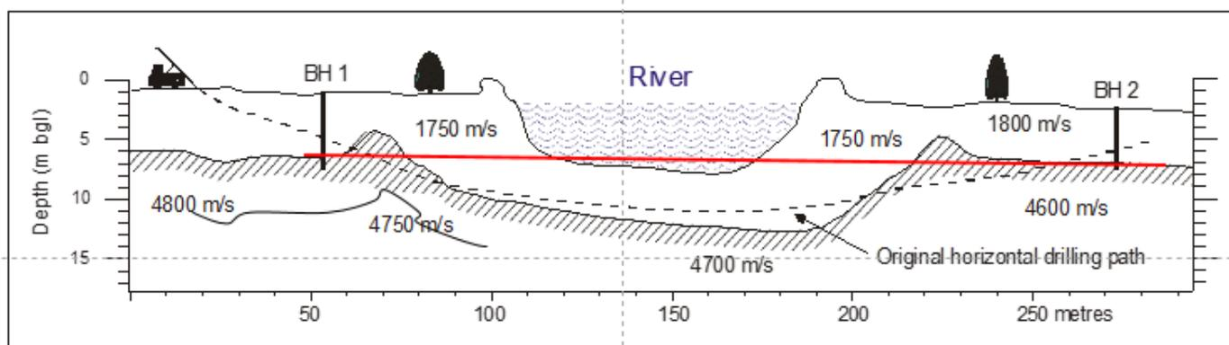
Figure 1: Schematic drawing of proposed Horizontal Directional Drilled (HDD) river crossing.
