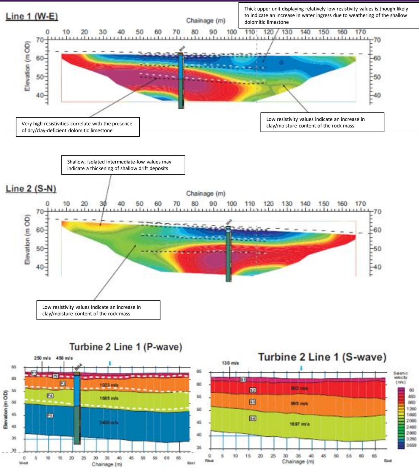
Figure 4: Geophysical results from one turbine location (Turbine 2) with (a) showing seismic refraction cross-section and (b) resistivity section
