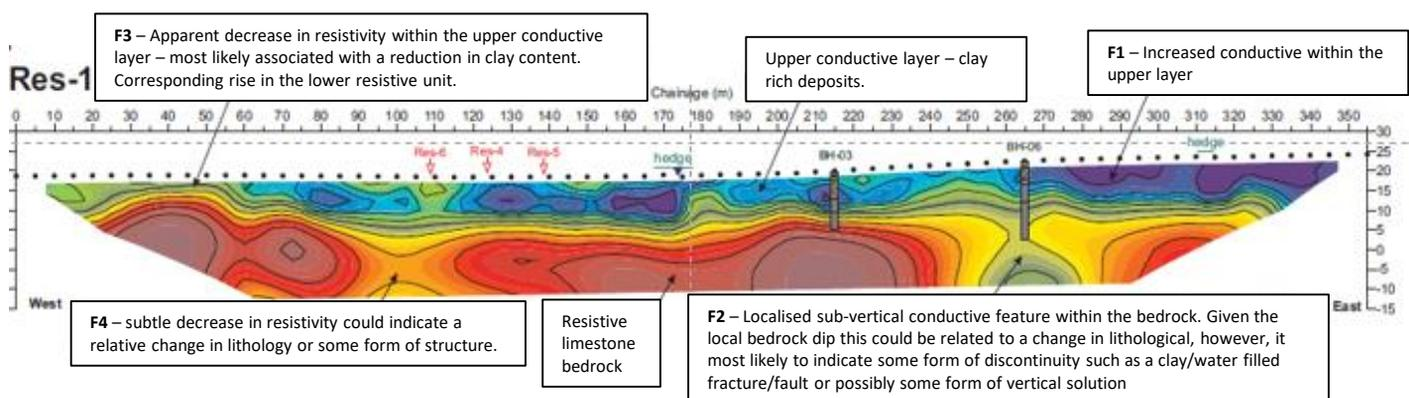
**Figure 3: Resistivity cross-section**
