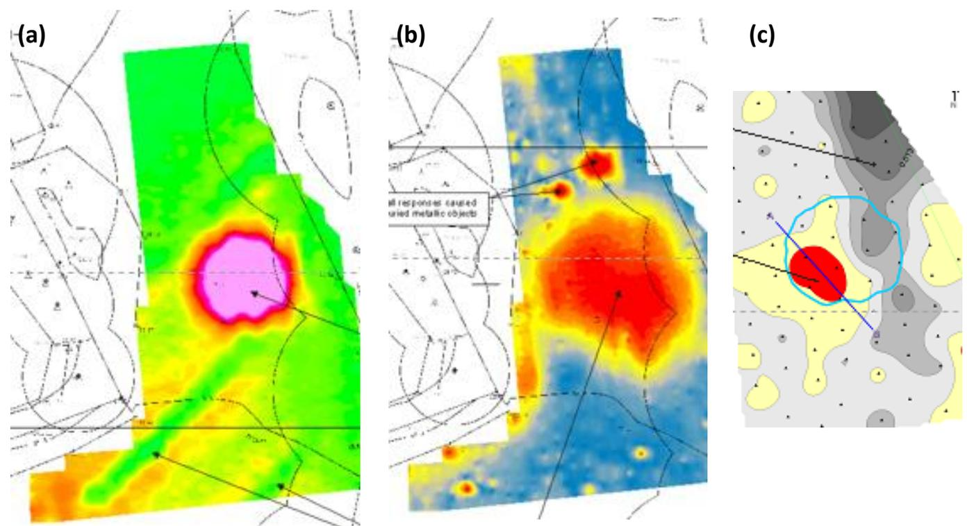
**Figure 2: Example results of (a) conductivity, (b) magnetic and (c) microgravity surveys**
