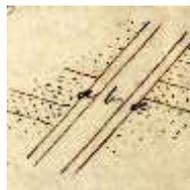
A Dyke disarranges the regularity of the Strata. Any Stratum on one side of the Dyke is lost at the Sticking, and on the same Level on the contrary side another Stratum presents itself which laid considerably above or below the Stratum on that side it was lost. When a Stratum lost on one side of a Dyke is found on [margin note – An Upthro [sic] Dyke] the contrary side above its Level that Dyke is called an Upthro [sic].
