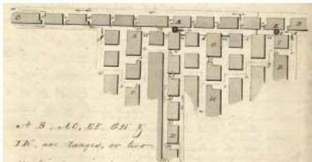
At **B, A C, E E, G H & I K**, are ranges, or two workings going parallel, between which there are Cross Workings **a, b, c, d** &c, made narrow at one end, These Cross workings are named Thirls. All the Thirls in each range are made up except that one next the foreheads of the Range. Ranges are meant to carry the
