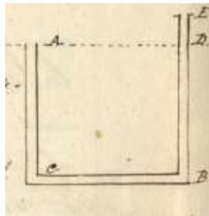
Thus suppose any Pit **A C**, the Air will be rarer at **C** than at **A**, if the Pit communicates with another **B D E**, and if that pit top is continued above the other Pit top any distance **D E** ‘till the Air at that part be as rare
