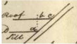
direction **d e** towards the Sill the Coal is sure to be found below on the other side of the Dyke
