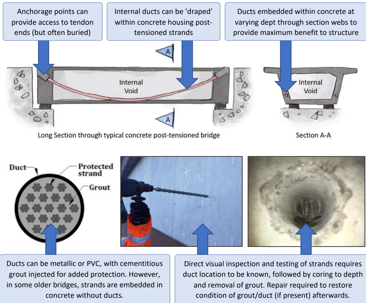
Figure 2 - Typical Post-Tensioned Duct/Strand Layout within Bridge and Intrusive Investigations
